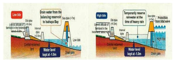
Fig. 2.8 The function of the sea dyke in the reclamation project Source: Isahaya Bay reclamation breakwater control office (Data accessed: 5<sup>th</sup> August, 2013)
