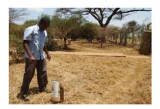
Figure 2. A rain gauge near the KWS headquarters (Picture in Amboseli NP)
