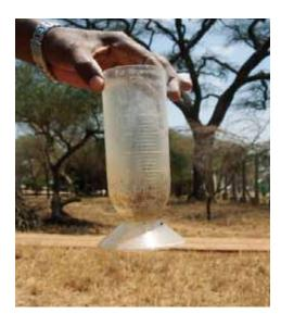
Figure 3. Inside cup of rain gauge (Picture in Amboseli NP)
